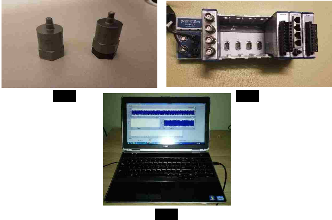
Figure 3.2: Components of Data Acquisition system: a) Accelerometers b) NI DAQ c) Computer with LabVIEW
